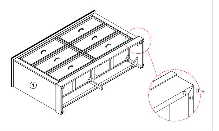
STEP 2: Attach Mirror leg ( 3 ) to Mirror ( 2 ) and Dresser ( 1 ) with bolt ( A ) and Flat washer ( B ), tighten it up by using an allen key ( C ).
